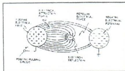
Figure 1-3. Voltage Potential Difference
