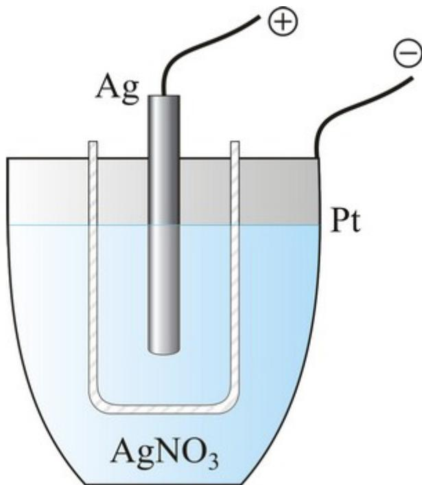
A **silver coulometer** is a device used to measure the quantity of electricity (in coulombs) by observing the amount of silver deposited or dissolved in a solution. Here's how voltage influences ions in the operation of a silver coulometer:
