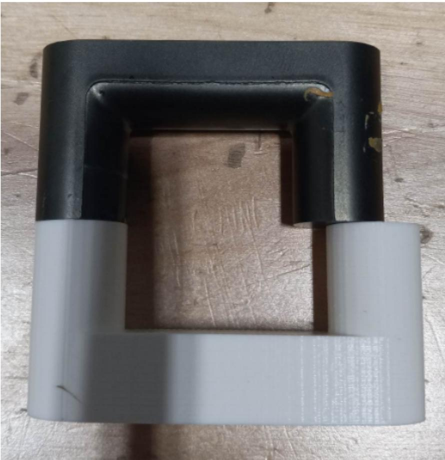
In the interest of making these core differences work out, I have redesigned the provided bobbin half pieces. Below is a link to the STL for 3D printing if you're so inclined to have purchased one of these cores. Please note that the thicknesses is 0.31". May need filing so core can fully meet together. 0.01" may be removed from each half piece center joining point.
