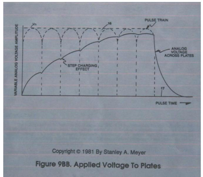
"Figure 9B. Variable Amplitude unipolar-pulse voltage frequency superimposed onto a 50% duty-cycle pulse-train."
