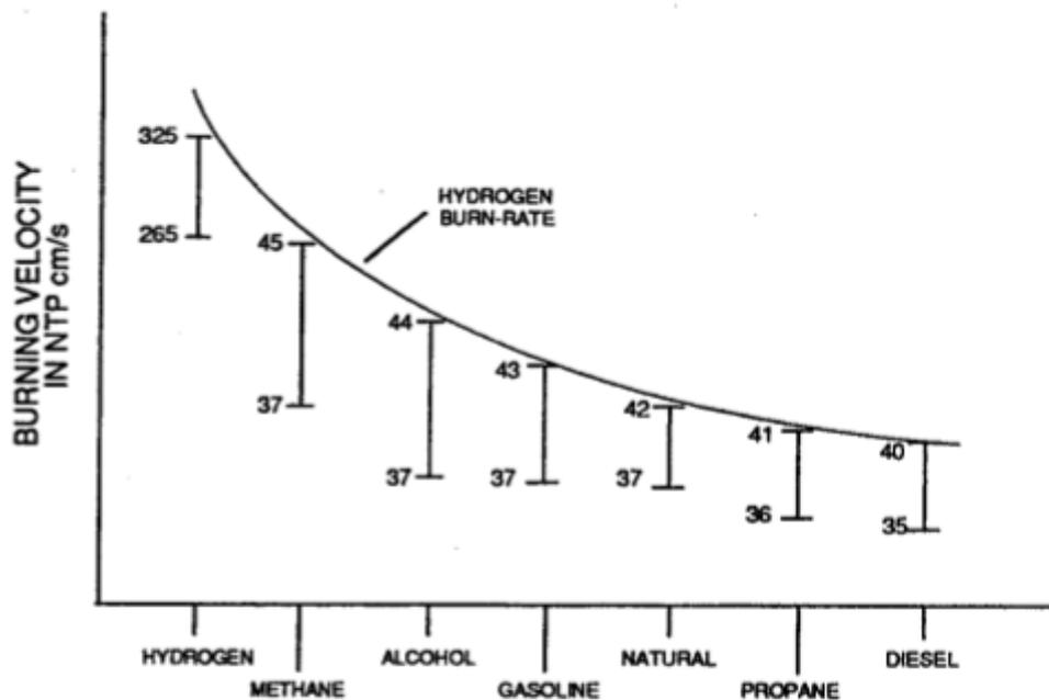
FIGURE 2-2: HYDROGEN BURN RATE
