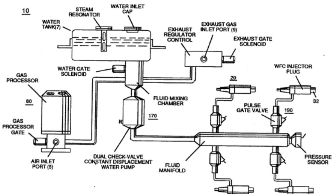
FIGURE 4-1: WATER FUEL INJECTOR SYSTEM
