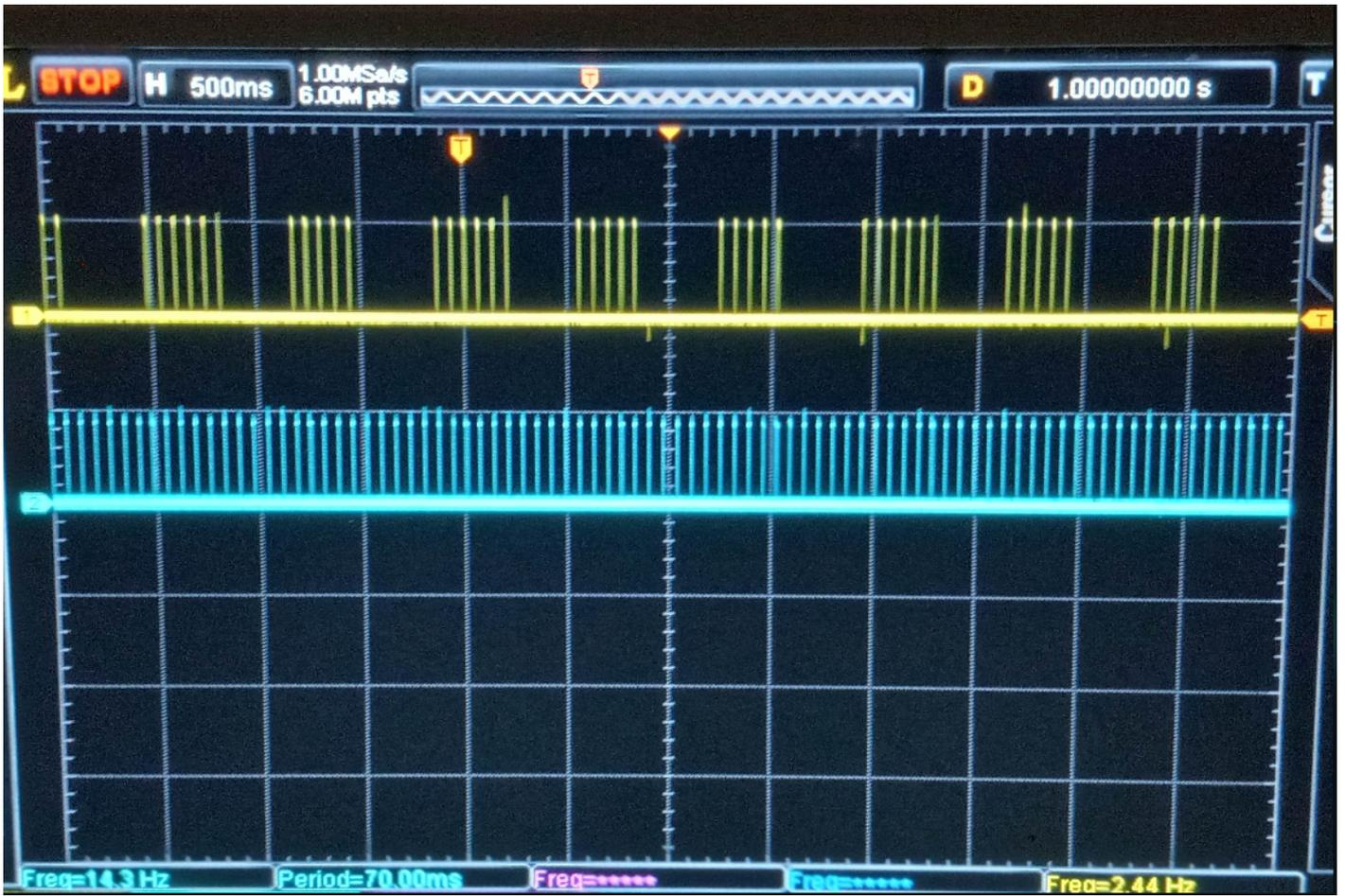
Pulse duty cycle ON time, down to lowest, measured at 1mS.
