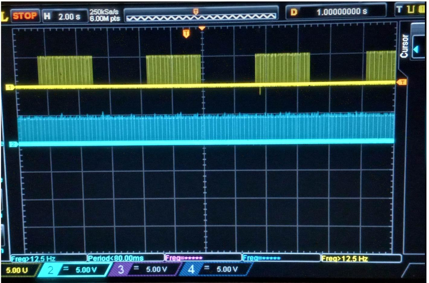
Gate can be adjusted by RA resistor to produce increase occurrences of pulse train
